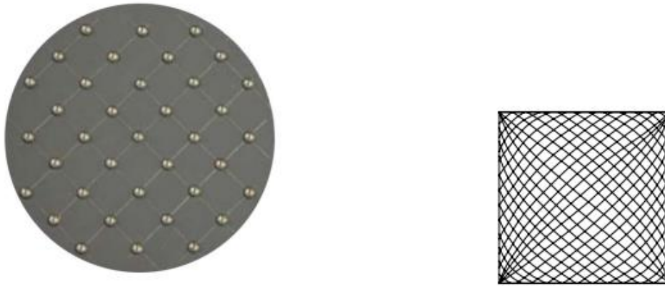
2-rasm - Lissajous figurasiga nisbatan shar plastinkasining yo'nalishi
